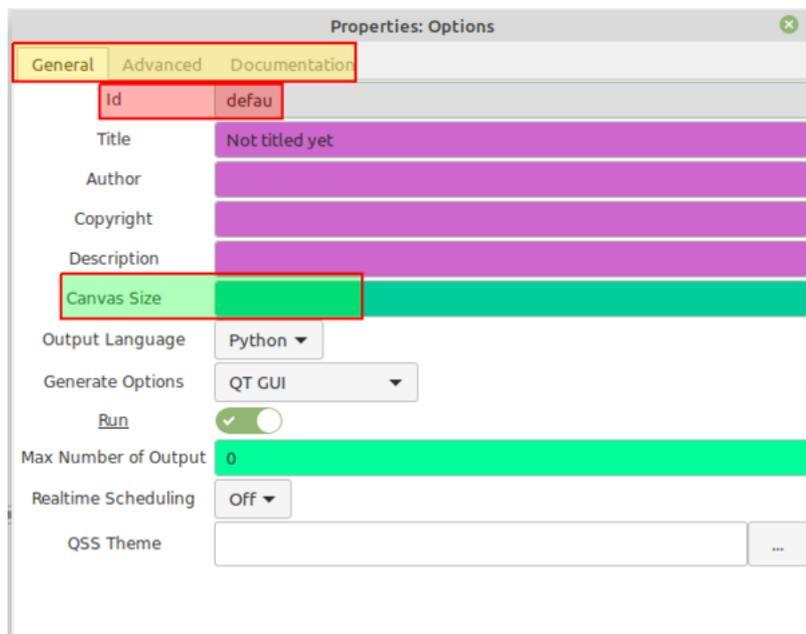
These block properties can be changed from the defaults to accomplish different tasks. Let's remove part of the current name and notice the **ID turns blue**. This color means that the information has been edited, but has not been saved. If we go back to
