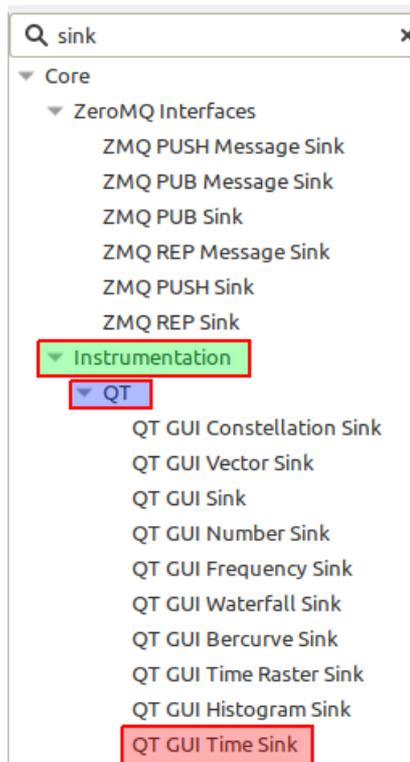
For now, let's add the block called **QT GUI Time Sink** by clicking on its name and dragging it to the Workspace or double-clicking on its name for it to be placed automatically in the Workspace.
