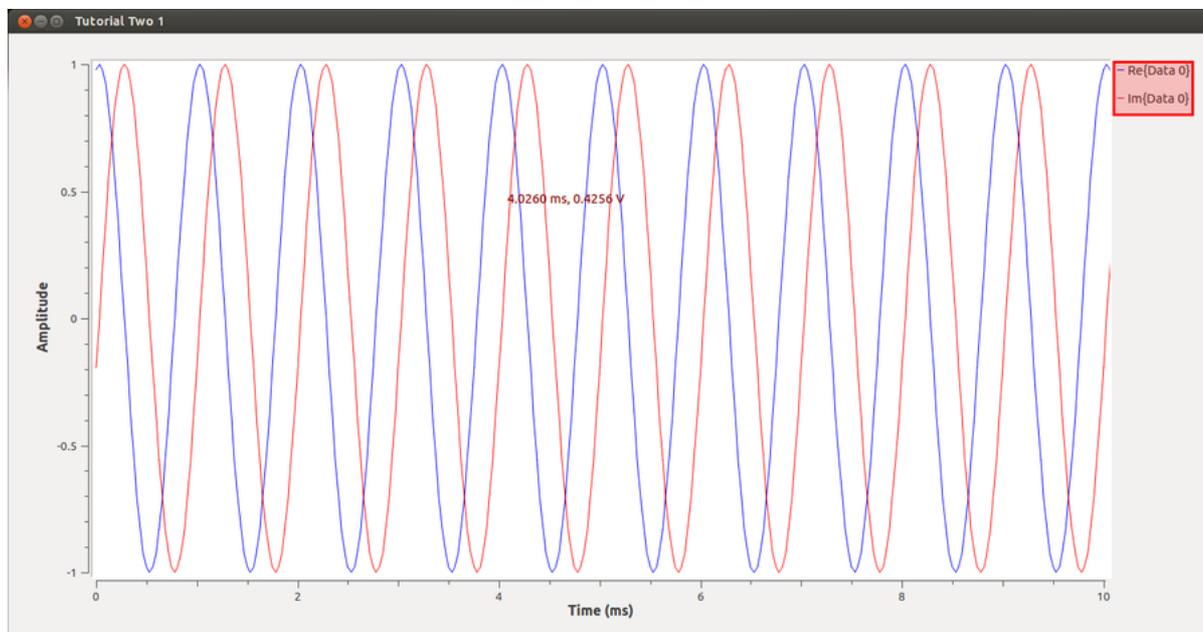
We should get the above which is a complex sinusoid of the form  $e^{j\omega t}$ . Let us keep things simple by avoiding complex signals for now. First we want to kill the flowgraph with the **Kill** flowgraph button or by simply closing the **Time Sink** GUI. Now is a good time to go over data types in GNU Radio by opening up the **Help->Types** window.
