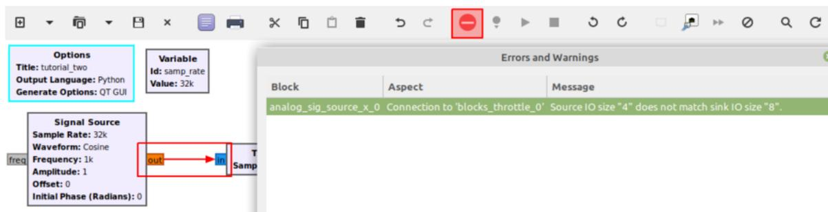
We see that **in the specified connection, there is size mismatch**. This is due to our data type size mismatch. GNU Radio will not allow us to chain together blocks of different data sizes, so let's change the data type of all of our subsequent blocks. We can now generate and execute as before. We now see our sine wave on one channel.
