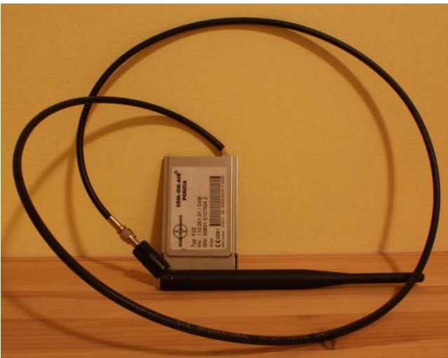
COA Type II with external antenna mod by Erik Tews
