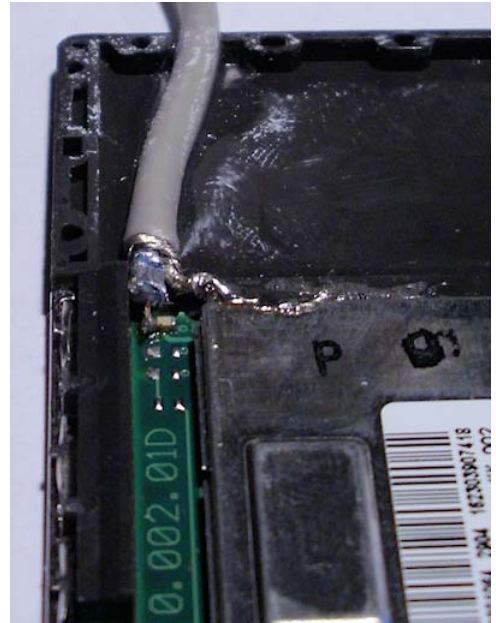
external antenna soldered (Tews)
