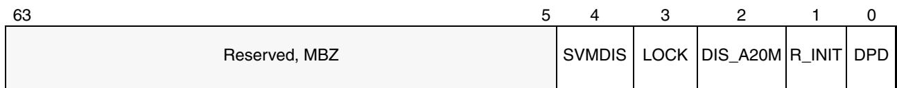
Figure 15-14. Layout of VM_CR MSR (C001_0114h)
