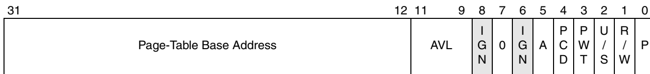
Figure 5-5. 4-Kbyte PDE—Non-PAE Paging Legacy-Mode
