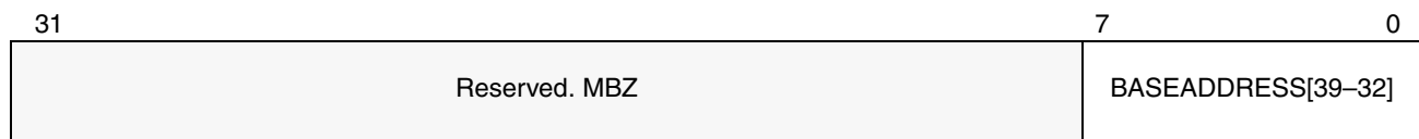
Figure 15-8. Format of DEV_BASE_HI[n] Registers
