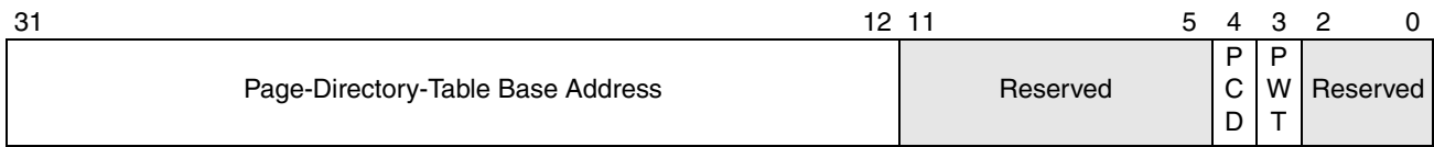
Figure 3-4. Control Register 3 (CR3)—Legacy-Mode Non-PAE Paging
