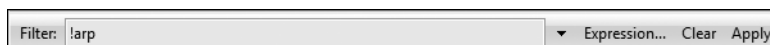
Figure 4-12: Creating a display filter using the Filter text box above the Packet List pane
