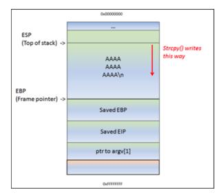
That means... If the data in [Buffer] is somewhat longer than 0x98 bytes, the strcpy() will overwrite saved EBP and eventually saved EIP (and so on). After all, it just continues to read & write until it reaches a null byte in the source location (in case of a string)
