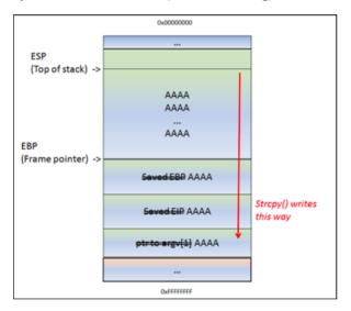
ESP still points at the begin of the string. The strcpy() completes as if nothing is wrong. After the strcpy(), the function ends. And this is where things get interesting. The function epilog kicks in. Basically, it will move ESP back to the location where saved EIP was stored, and it will issue a RET. It will take the pointer (AAAA or 0x41414141 in our case, since it got overwritten), and will jump to that address.
