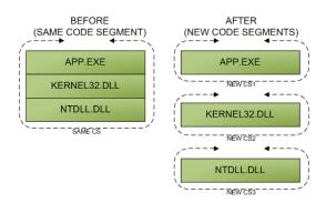
Figure 2: Not-encapsulated and encapsulated modules inside of the process memory.
