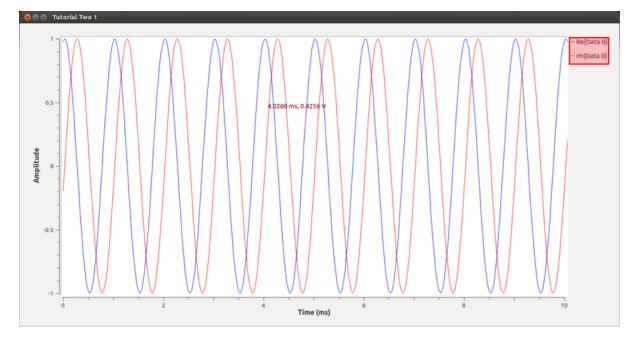
We should get the above which is a complex sinusoid of the form e <sup>jwt</sup>. Let us keep things simple by avoiding complex signals for now. First we want to kill the flowgraph with the **Kill** flowgraph button or by simply closing the **Time Sink** GUI. Now is a good time to go over data types in GNU Radio by opening up the **Help->Types** window.
