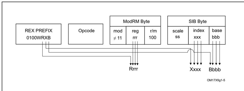
**Figure 2-5. Memory Addressing With a SIB Byte**
