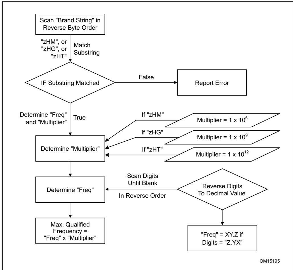
**Figure 3-9. Algorithm for Extracting Maximum Processor Frequency**
